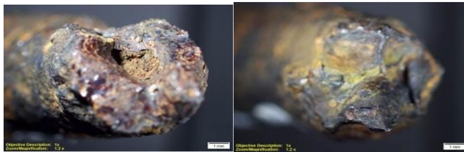
Figure 6. Fracture surface of a broken spring sample D which experienced ductile fracture.
