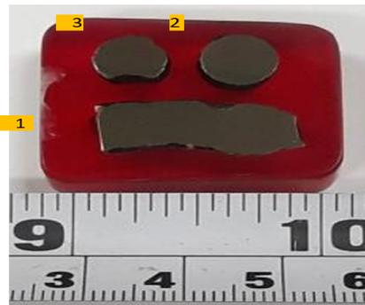
Figure 9. Location of Etched and Non-Etched Metallographic Examination of Spring Sample A
