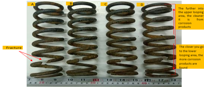
Figure 1. Visual material identification carried out on broken springs
