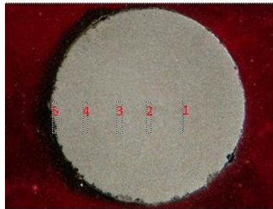
Figure 23 Location of Cross-Section Hardness Test of Whole Spring
