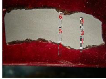
Figure 22 Location of Longitudinal Section Hardness Test for Broken Spring
