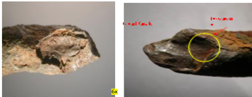
Figure 3. Fracture surface of spring sample A which experienced ductile fracture
