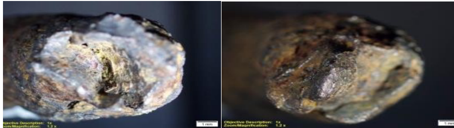
Figure 5. Fracture surface of broken spring sample C which experienced ductile fracture
