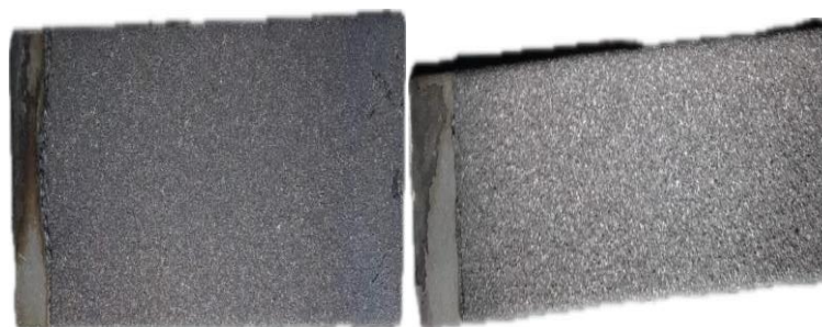
Image 2. Coating 95 MXC (top), coating SS420 (below)
