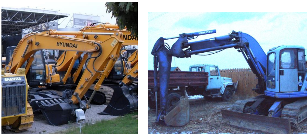
Figure 1.15 - Mounting options for the hydraulic cylinder of the handle of the single-bucket hydroficated DSM.
