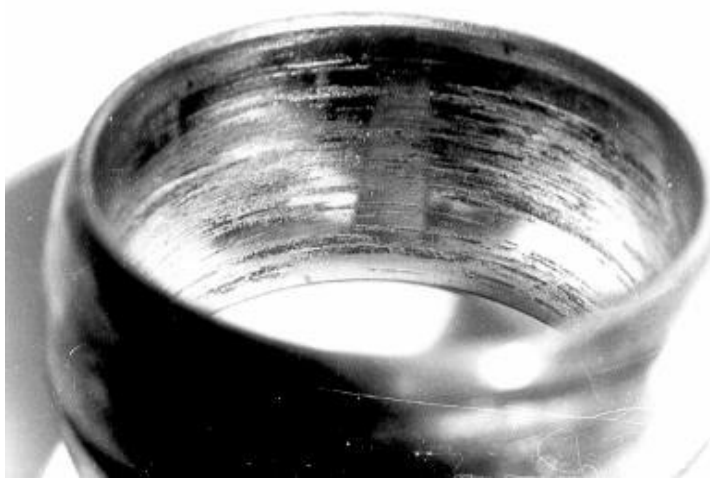
Figure 1.10 - Worn surface of the lug spherical bearing element.
