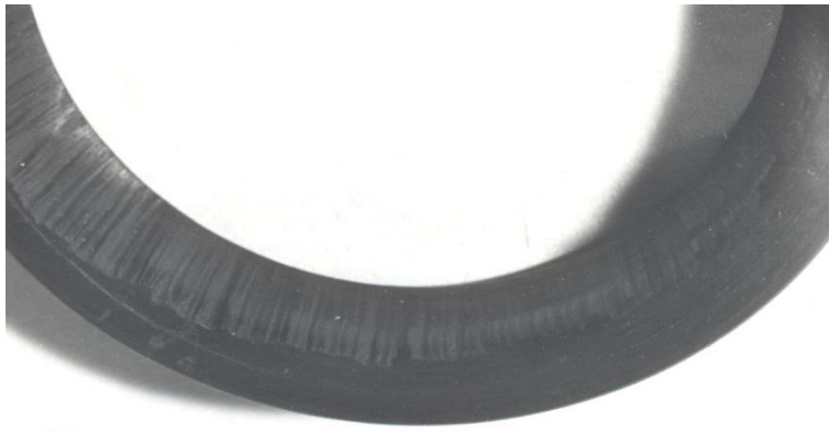
Figure 1.9 - Characteristic wear of the seal.
