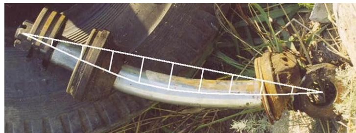
Figure 1.8 - Curvature of the rods.
