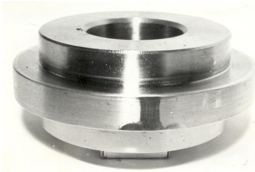
Figure 1.7 - Characteristic wear of the piston surface in the initial period of running-in of interface elements.
