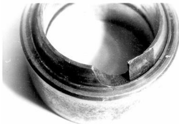
Figure 1.11 - Partial destruction of the element of the spherical bearing of the eye of the rod.
