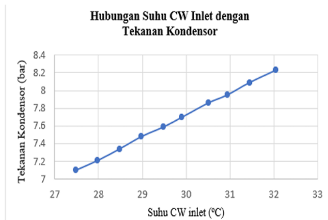
Figure 4. Graph of the Relationship Between Cooling Water (CW) Inlet Temperature and Condenser Pressure at 80% Cooling Load
