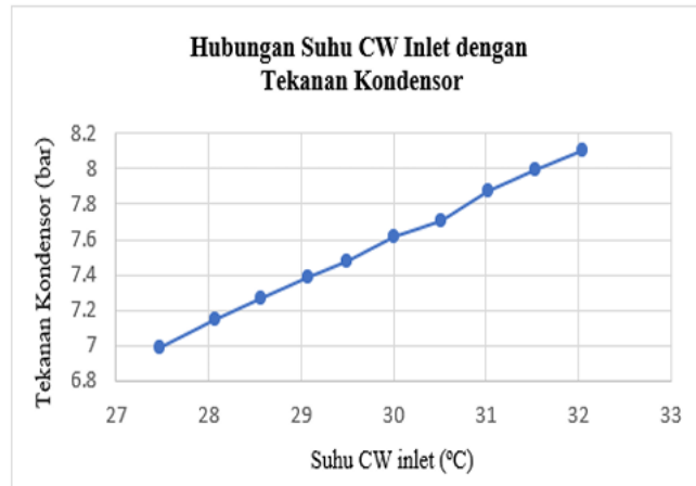
Figure 3. Graph of the Relationship Between Cooling Water (CW) Inlet Temperature and Condenser Pressure at 72% Cooling Load
