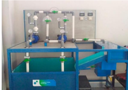
Figure 5. Centrifugal Pump Series Based on Characteristics
