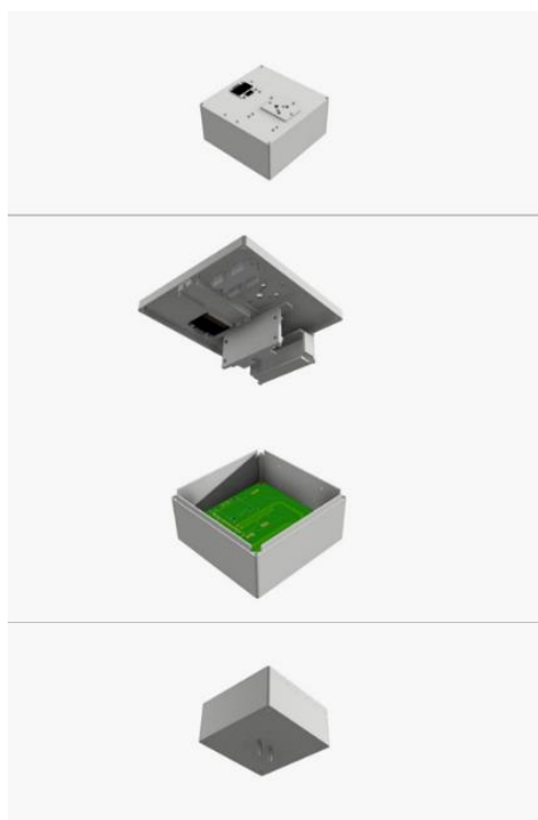
Fig. 8. 3D Print Design for The Device Casing
