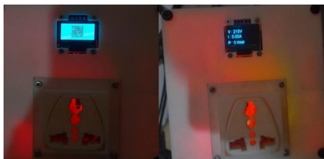
Fig.9. Show the QR Code and the measurements on Oled
