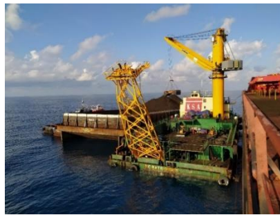
Figure 1 Coal loading and unloading activities from barges to ships using floating cranes
